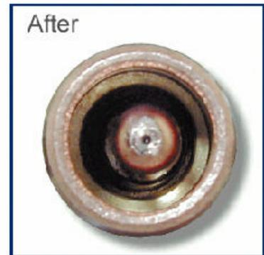
The IWE UltraCleaner is the first non-mechanical cleaner that can automatically remove spatter from any robotic GMAW torch including twin wire. The ultrasonic waves created in the anti-spatter fluid remove spatter from all torch components; including the contact tip, diffuser and nozzle. Longer consumable life is obtained because the UltraCleaner **cools as it cleans**.
